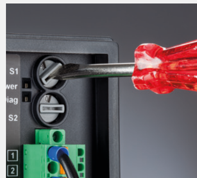
Input ranges and floating standard-signal output selectable
